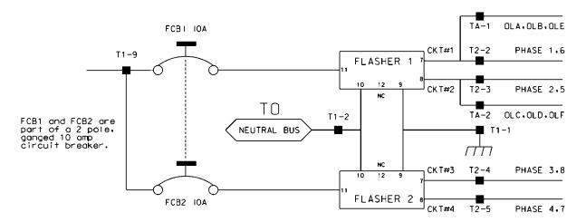
Ensure auxiliary output files are wired as follows:
